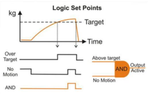
R400 Logic set points are based on the status of the inputs and the defined mask that is used to match IO1-IO24 for the logic set points.
